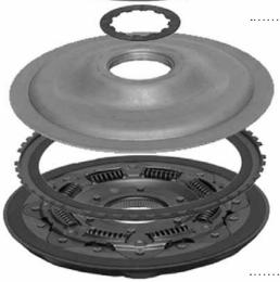
Only the lowest stall impellers are used to manufacture these converters. The impellers used are even lower stall than the typical low stall 'straight rib' impellers; only impellers that have an extra 'low stall' negative rib angle are utilized in building these part numbers. All impellers are manually or furnace brazed for added
