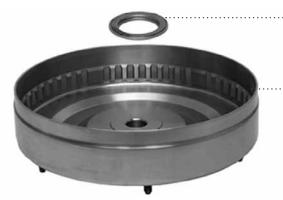
Bearing between the turbine hub and front cover is also 'latest design'. Replaced 100%, this bearing has a 'shoulder' that keeps the race properly positioned in all phases of converter operation.
