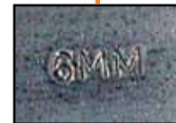
"6MM" or "WW9" metal stamped in cover
