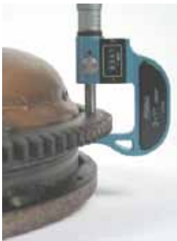
Measuring the thickness of the ring gear
