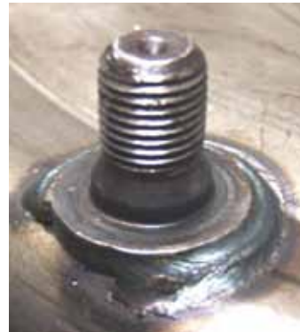
FIG 2. Stud with tapered base. Stud does not have threads all the way to the base. Stud flares out to approximately .470" at base.
