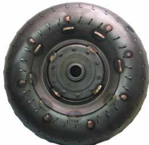
Upgraded turbine w/ reinforcing plate welded in place
